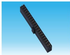
2.54mm Female Header, Dual Row, Straddle
